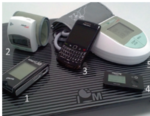
Fig. 2: The first generation of the measuring devices connected to CO-MES® to be used as Virtual Lab equipment: 1) blood glucose meter; 2) wrist sphygmomanometer; 3) Blackberry telephone with Bluetooth connection; 4) step counter; 5) upper arm sphygmomanometer
