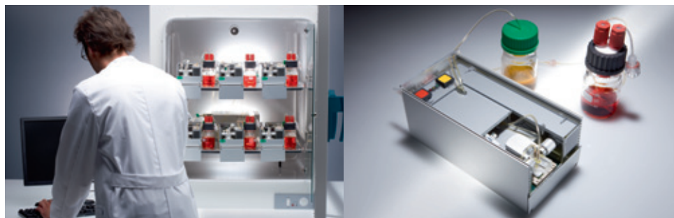
Fig. 3: The 6xIMOLA-IVD device enables examination of six cell samples at the same time. For optimum temperature control, the system is integrated into an incubator.
