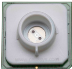
Fig. 1: BioChip-C (side length: 24 mm) with two pH sensors, two bioimpedance sensors, a sensor for measuring dissolved oxygen, a temperature sensor and various test electrodes.
