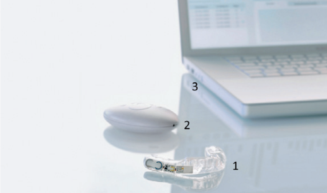
Fig. 2: Complete system including: occlusal splint (1); tactile biofeedback system (2); front-end computer (3)
