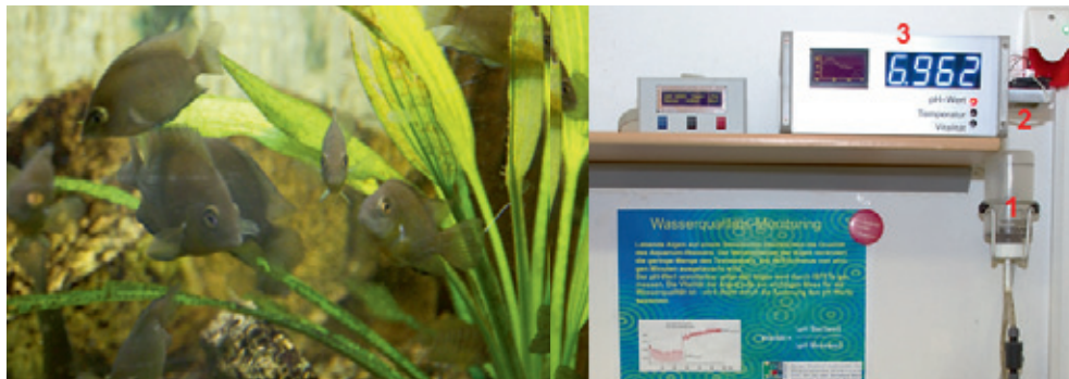
Fig. 3: Monitoring of water quality: (1) Aquarium water inflow and outflow; (2) Sensor module with pH-ISFETs, algae culture on silicon sensor chips and LED light source for ensuring photosynthesis; (3) Electronic unit for the pH-ISFETs with data display.
